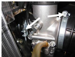
• Re-fill the float chamber by pressing the fuel in the syringe into the float chamber.
