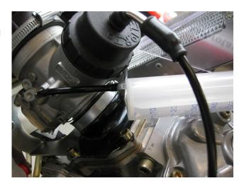
• Turn the carburettor towards the seat in horizontal position.
