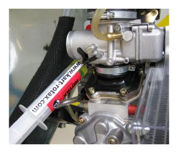
Remove the carburettor plug screw, change the main jet and fit the carburettor plug screw again.
