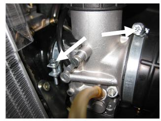
Connect the syringe (60 ml, ROTAX part no. 581 385) with the left hole of the venting tube.
