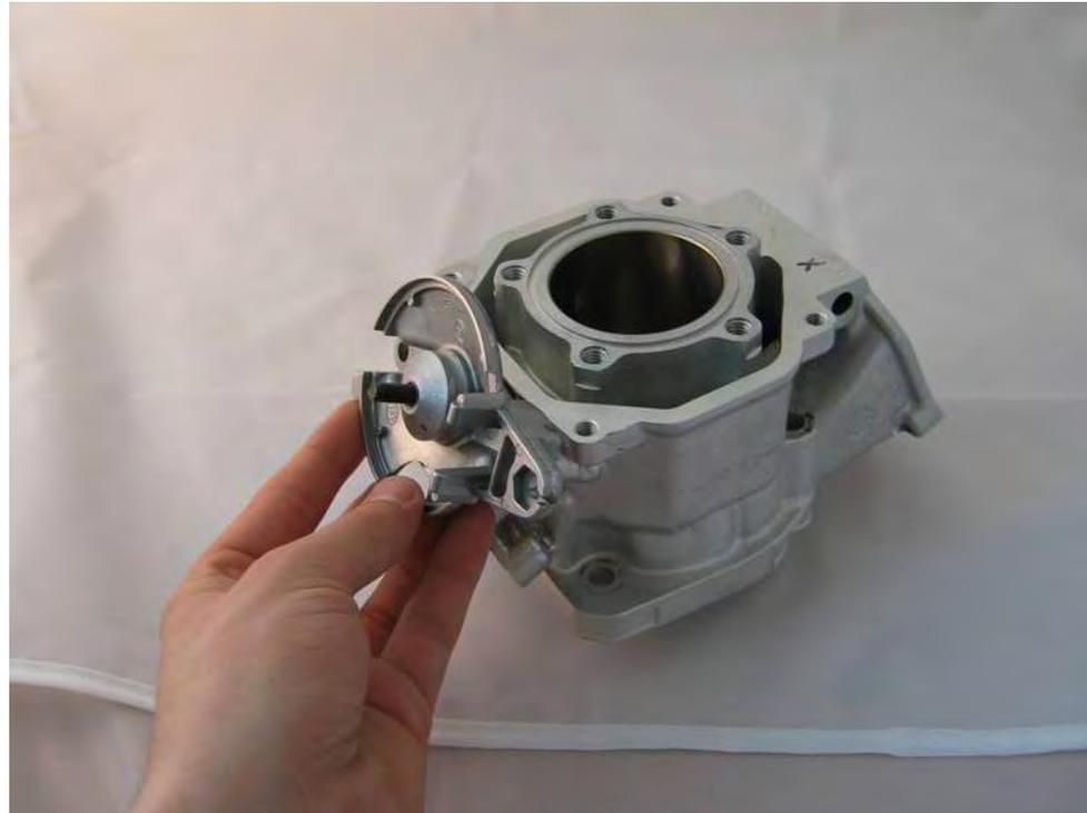
Apply the valve rod housing to the cylinder and check the exhaust valve for free movement.
