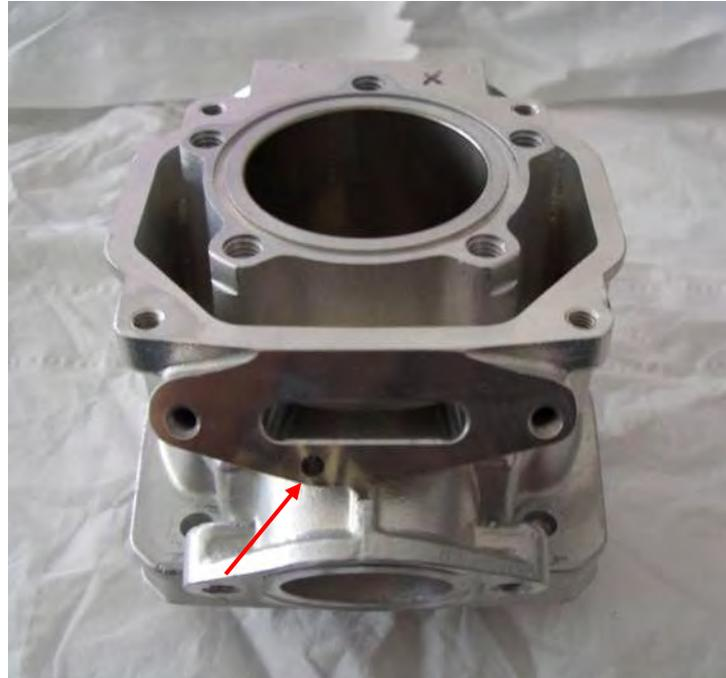
Clean the cylinder with brake cleaner and check impulse bore for cleanliness. (visual)
