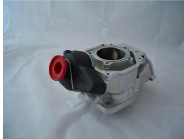
Apply the compression spring to the Exhaust Valve and mount the Valve Cover by means of the spring clip to the housing.
