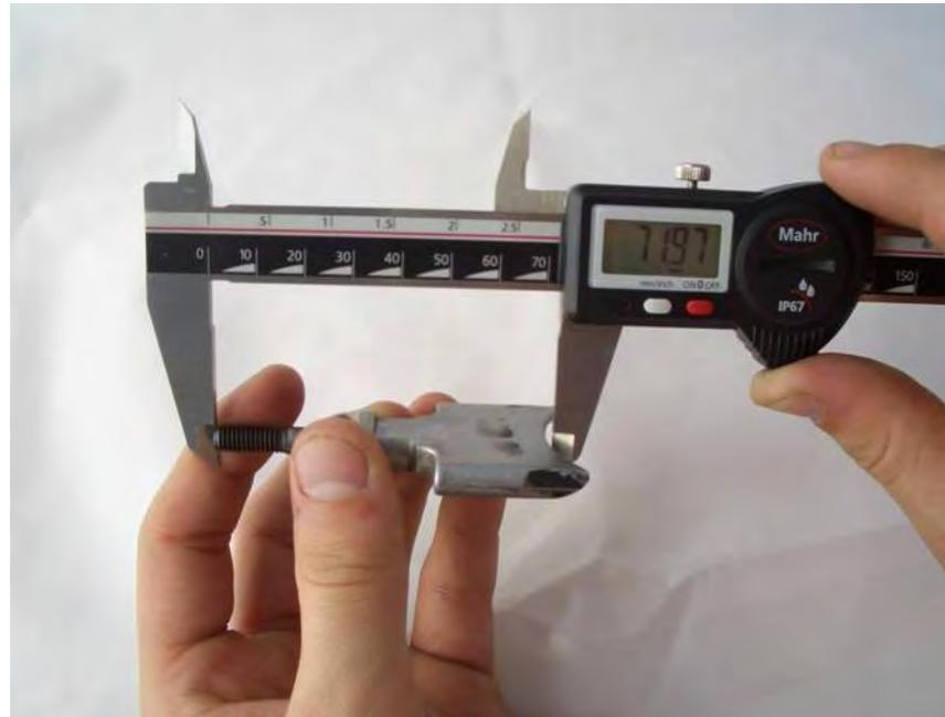
Clean the Exhaust valve with brake cleaner and scotch brite and check the total length of the exhaust valve. ( 72 +/- 0,3)
