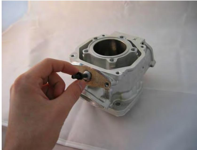
Apply the o-ring to the stud screw.
