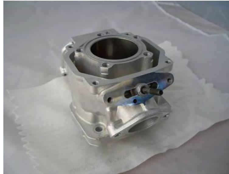
Insert the exhaust valve as shown on the picture and assure free movement of the exhaust valve.
